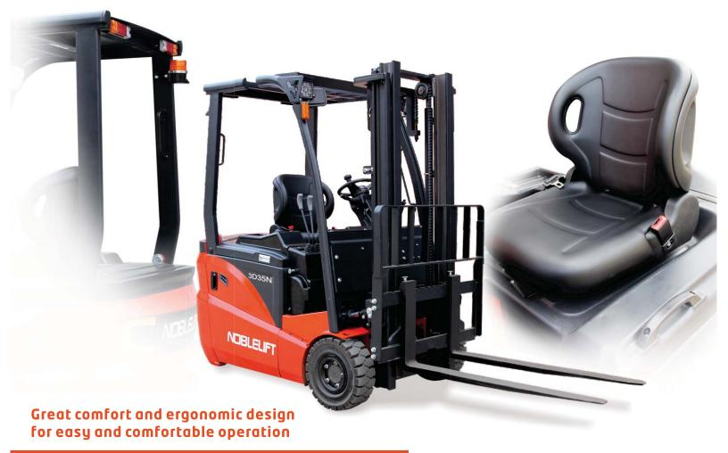
The N series is designed with full consideration of the comfort and ergonomic of the operator to ensure the best efficiency and productivity is delivered with easy and comfortable operation. All lights are LED to ensure the best view in dark areas. Small diameter steering wheel with spinner knob and on-demand Fully Hydrostatic Power Steering (FHPS) ensures effortless steering of the forklift during operation. Spacious step area with anti-slip design and a large hand grip for easy entry and exit.
